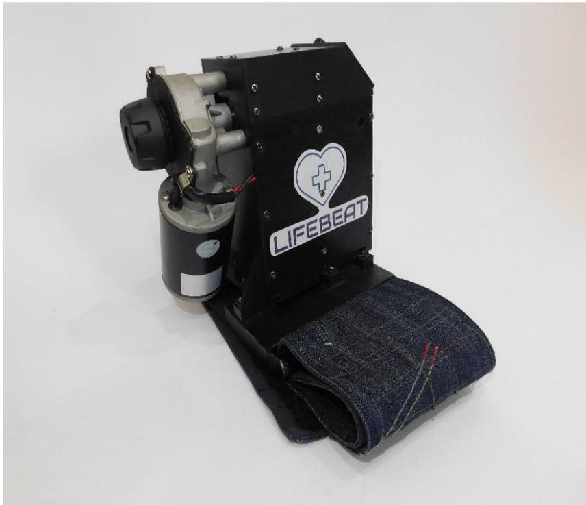
**Figure 8.** Chest compression device complete in its third phase
