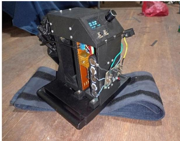
Figure 6. Complete chest compression equipment of the second phase
