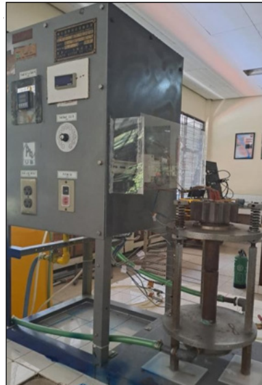
Figure 2. Thermal conductivity measuring device
