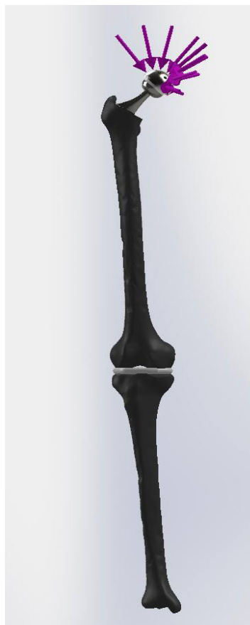
Figure 1. Model of the lower limb with a prosthetic head of the hip joint, the force vectors acting on the prosthesis are indicated
