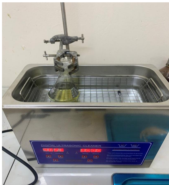
Figure 4. Shows the final step in preparing the nanomulsion using the ultrasonic water bath device
